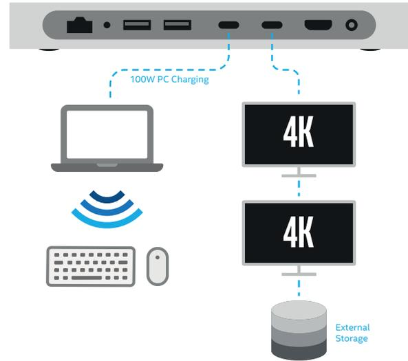
**Figure 2.** Thunderbolt 3 allows a single cable to provide more data and video bandwidth than any other cable, while also supplying power.
