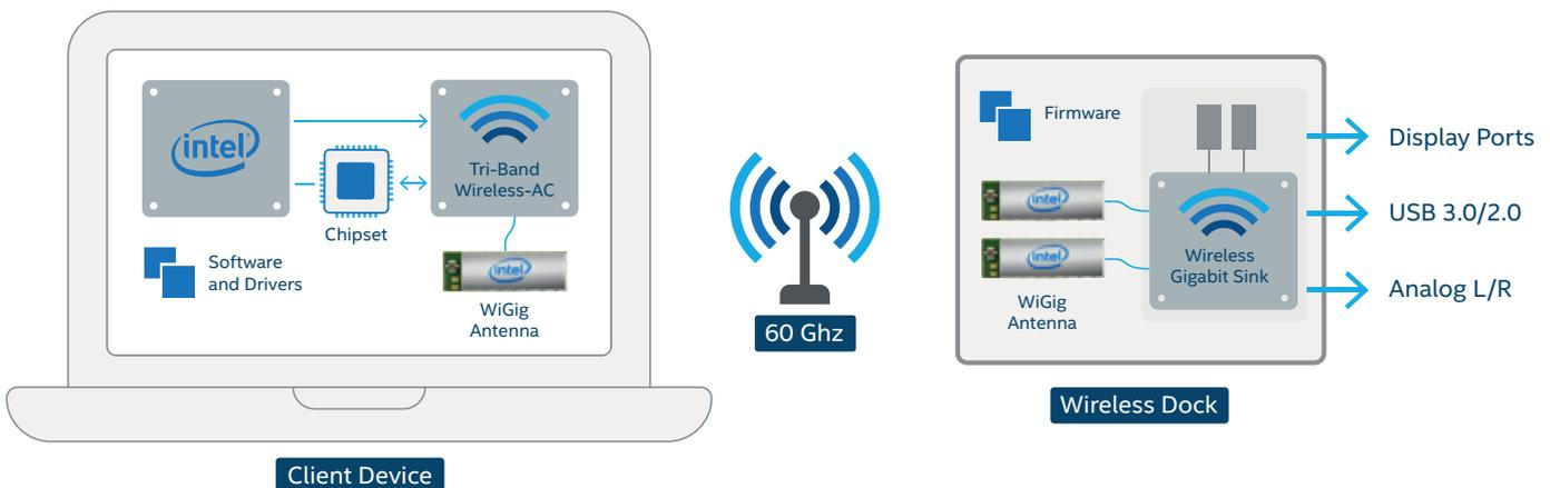
**Figure 1.** Intel Wireless Docking: Every component, from drivers and firmware to the silicon Tri-Band Wireless-AC module, antennas and dock “sink” chip, are developed and tested together to provide the best solution for the end-user.
